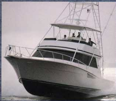
HER SHARP ENTRY AND FLARED BOW GIVE THE 53' HER UNCOMMONLY SOFT, DRY RIDE.
